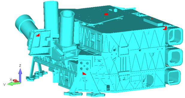
Figure 5: Sensor locations in the FEM (1/3)
