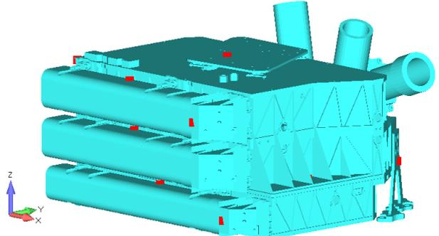
Figure 6: Sensor locations in the FEM (2/3)
