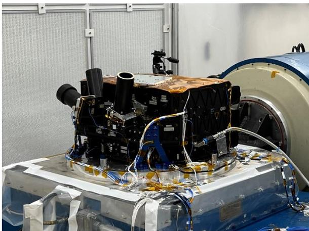
Figure 1: The ALTIUS Optical Unit instrument STM mounted on a shaker bench
