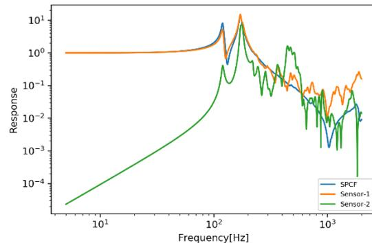
Figure 3: Example showing two sensors tracking the interface force. One of them (orange) has a much better correspondence with the interface force than the other (green)
