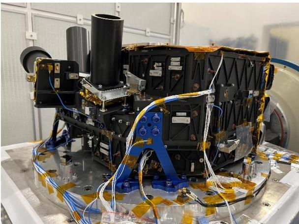
Figure 4: A close up of the ALTIUS OU instrument STM mounted on the shaker table with accelerometers
