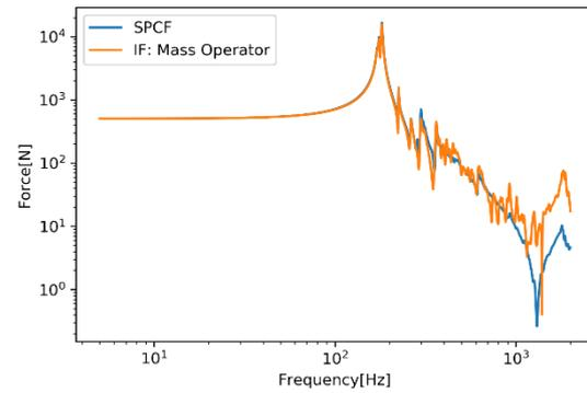
Figure 8: Comparison of the interface force calculated directly from the FEM (orange) and the interface force estimated through the mass operator method (blue)
