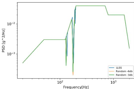
Figure 11: Differences in the analytically calculated notch profiles with revision of the interface loads.
