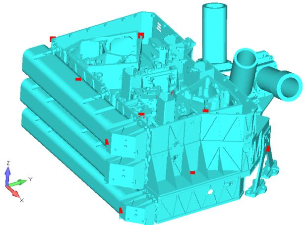
Figure 7: Sensor locations in the FEM (3/3)
